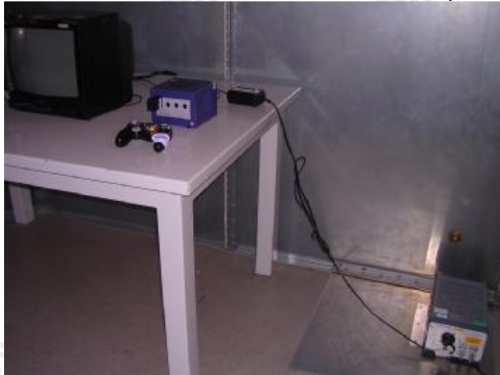
Measurement of Conducted Emission Test Set Up
