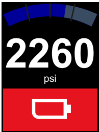
Fig. 16 Critical battery alarm
