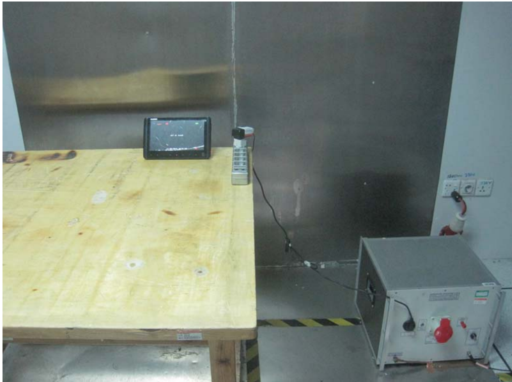
Photograph – Conducted Emission Test Setup
