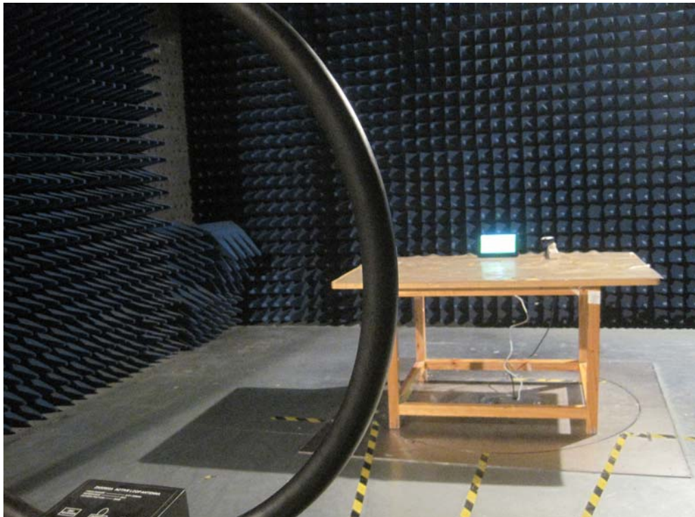
Photograph – Radiation Spurious Emission Test Setup
