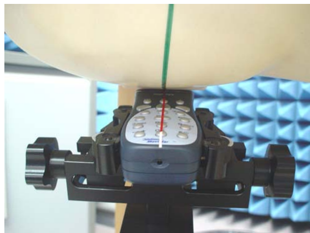
Fig.4 Right Head Section / Cheek-Touch Position
