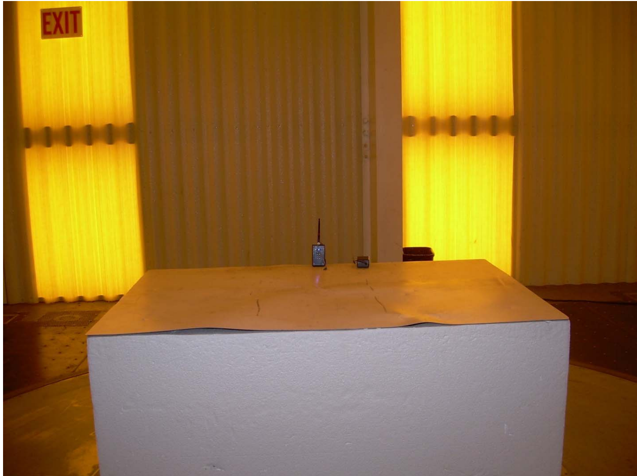
Photograph 1 – Front View Worst-Case Radiated Emissions Setup
