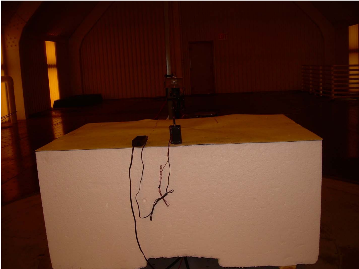
Photograph 2 – Front View Worst-Case Radiated Emissions Setup
