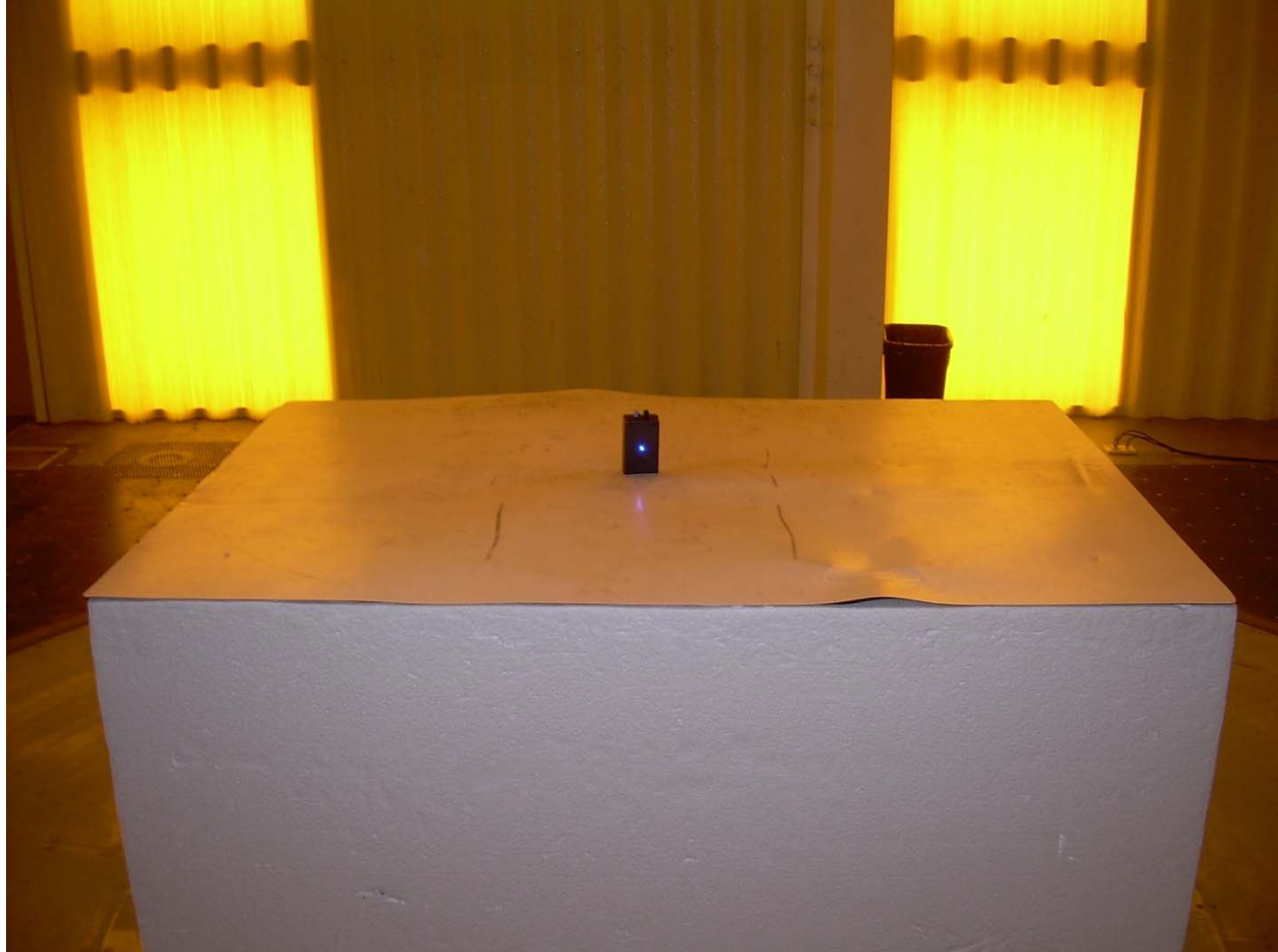
Photograph 1 – Front View Worst-Case Radiated Emissions Setup
