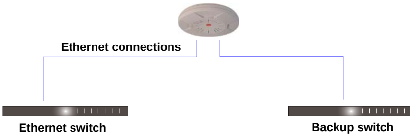
Figure 24. Switch Failover Protection
