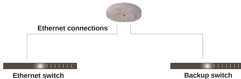
Figure 25. Switch Failover Protection
