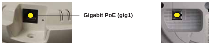
Figure 33. Network Interface Ports—XR-520 (left); XR-1000 Series (right)
