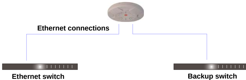
Figure 23. Switch Failover Protection
