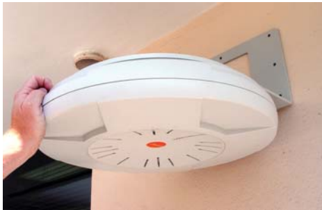
Figure 42. Mounting the Array on a Wall
