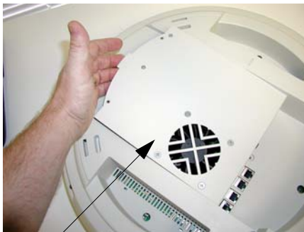
Access panel (with power supply and fan)
