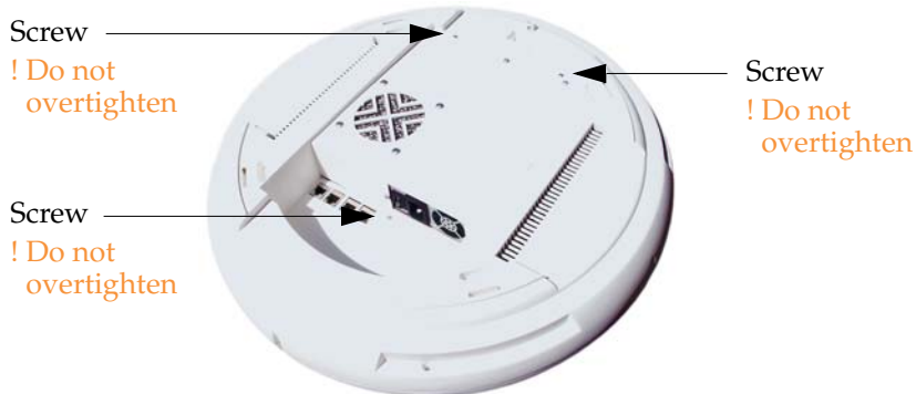
Figure 115. Reinstalling the Access Panel
