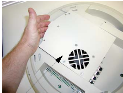
Access panel (with power supply and fan)
