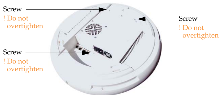
Figure 118. Reinstalling the Access Panel
