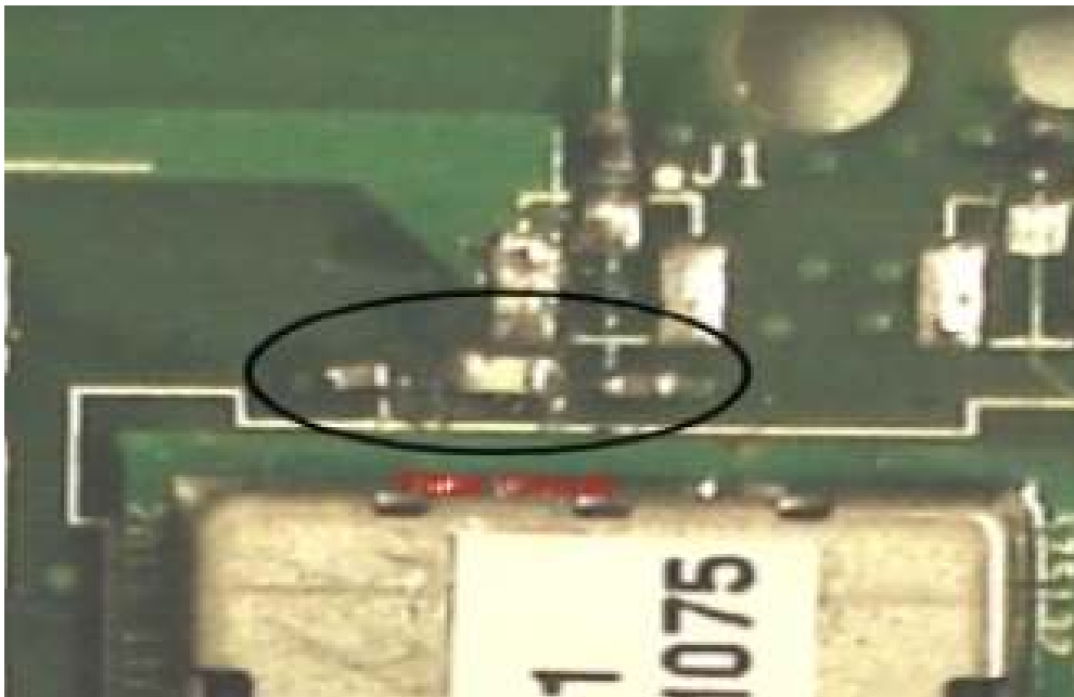
Component Side Zoom (Filter Circuit)
