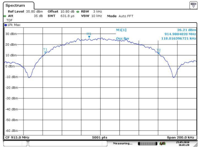
Figure 7.4.4.2-10: Sample Plot 99% OBW- DSSS – 12.5kbps
