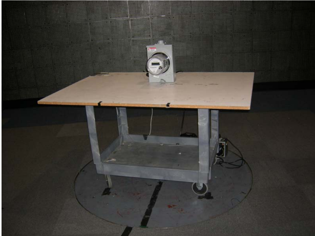
Figure 7: Test Setup – Radiated Emissions - Intentional
