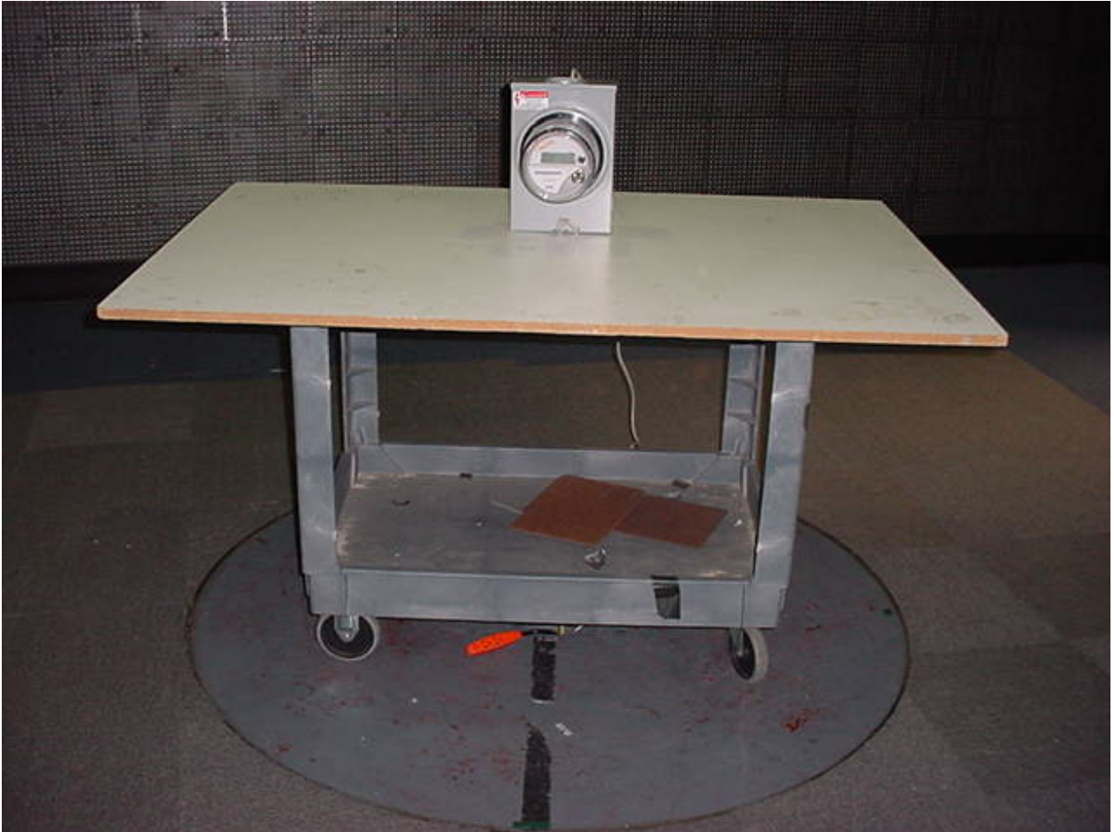
Figure 3: Test Setup – Radiated Emissions - Unintentional
