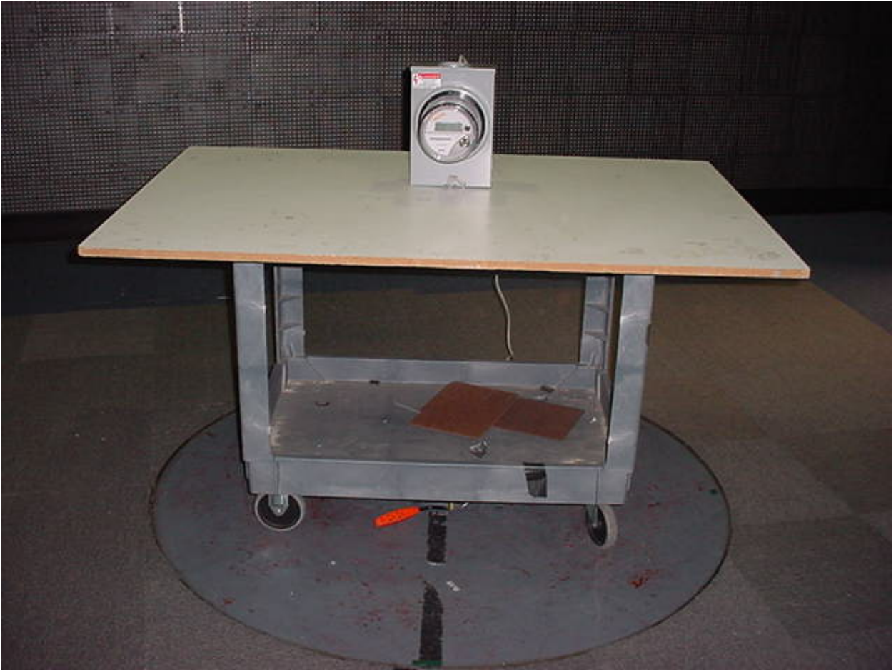
Figure 9: Test Setup – Radiated Emissions - Unintentional
