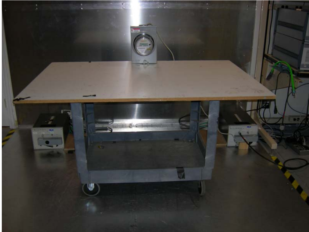
Figure 13: Test Setup – AC Power Line Conducted Emissions
