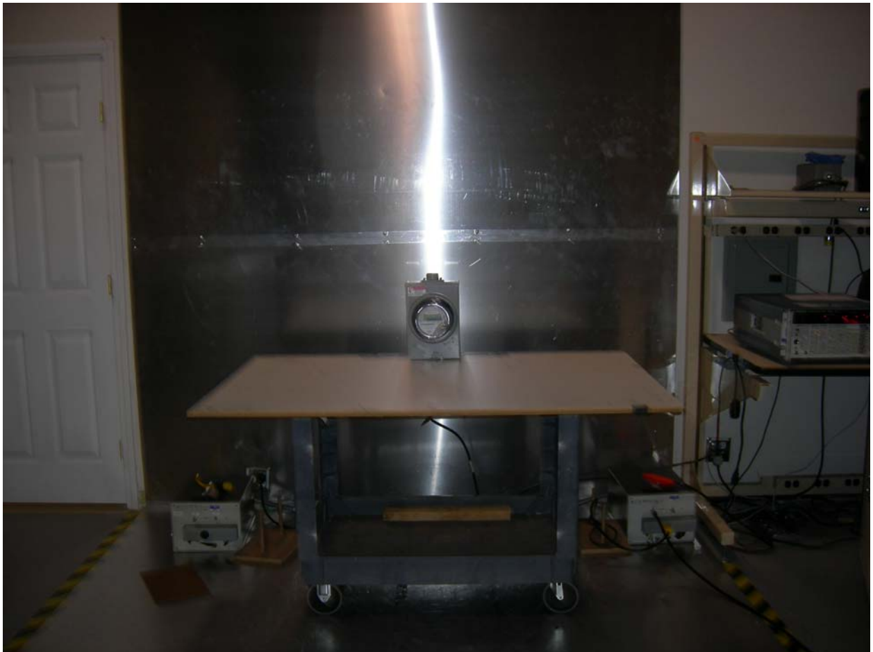
Figure 5: Test Setup – AC Power Line Conducted Emissions
