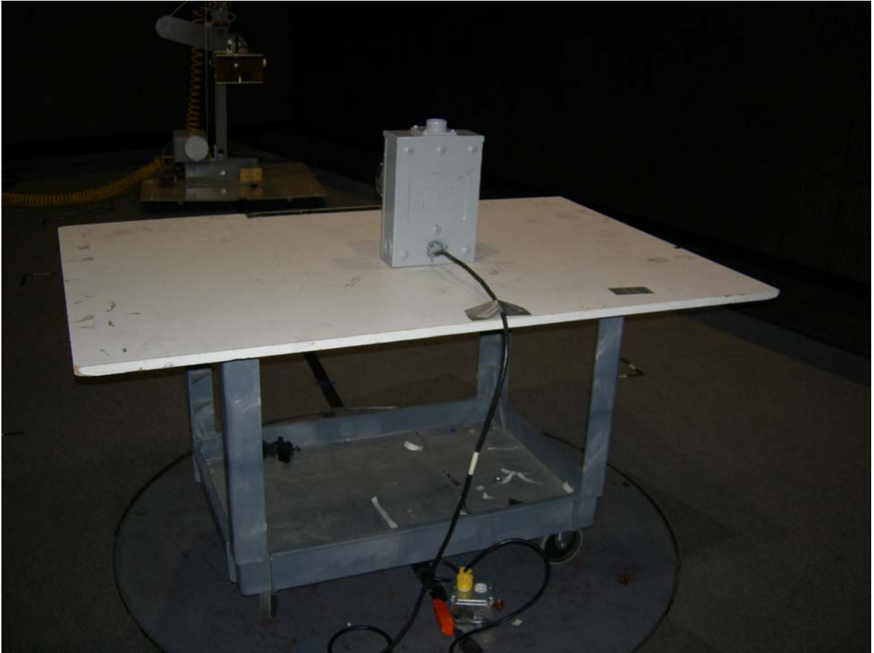
Figure 2: Test Setup – Radiated Emissions - Intentional
