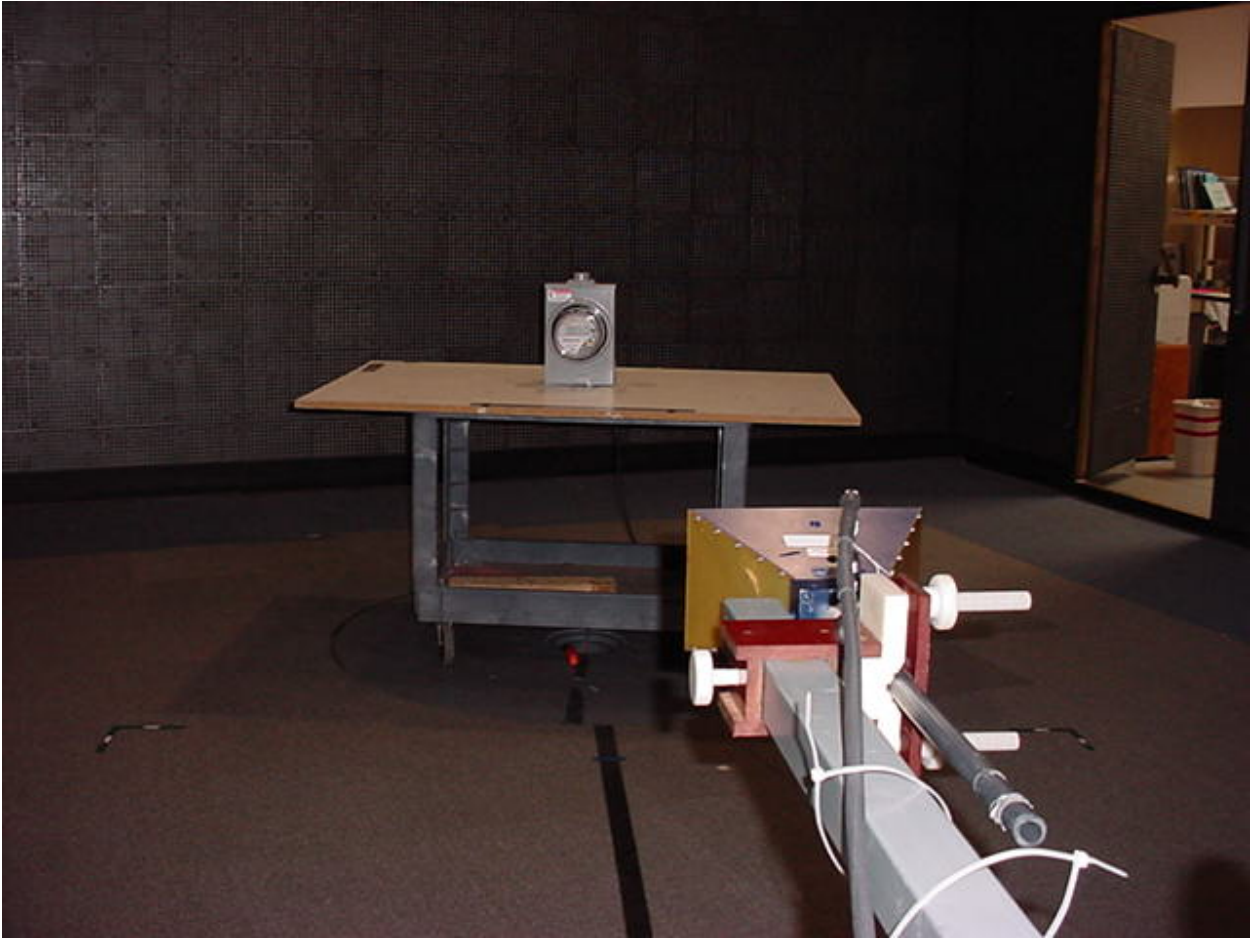
Figure 8: Test Setup – Radiated Emissions - Intentional
