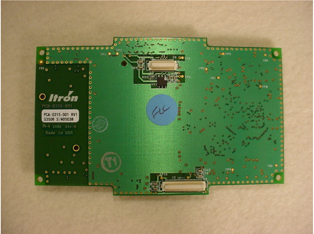
Figure 9: Internal – Mezzanine GPRS Modem Board Back
