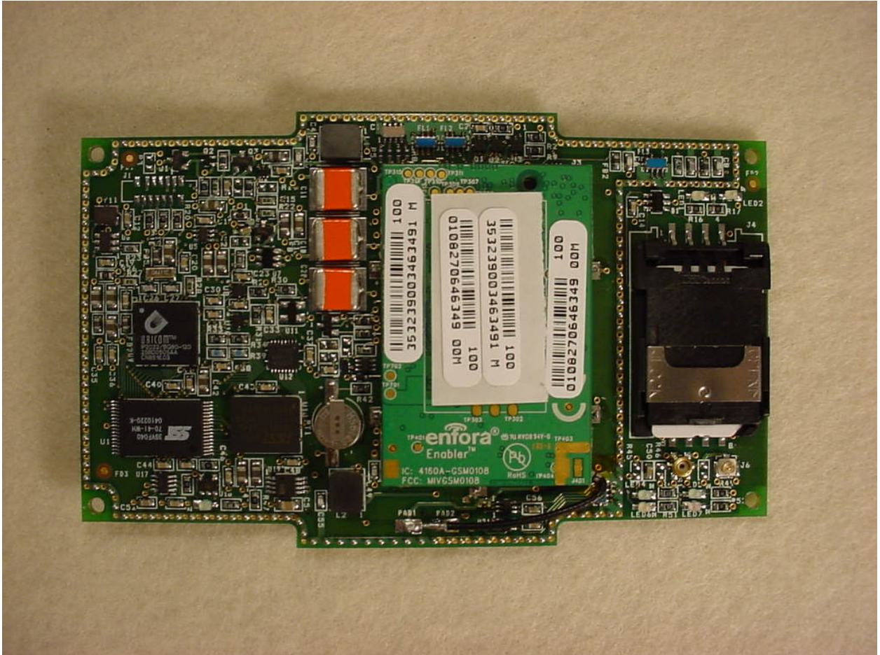
Figure 7: Internal – Mezzanine GPRS Board Front w/o Shields
