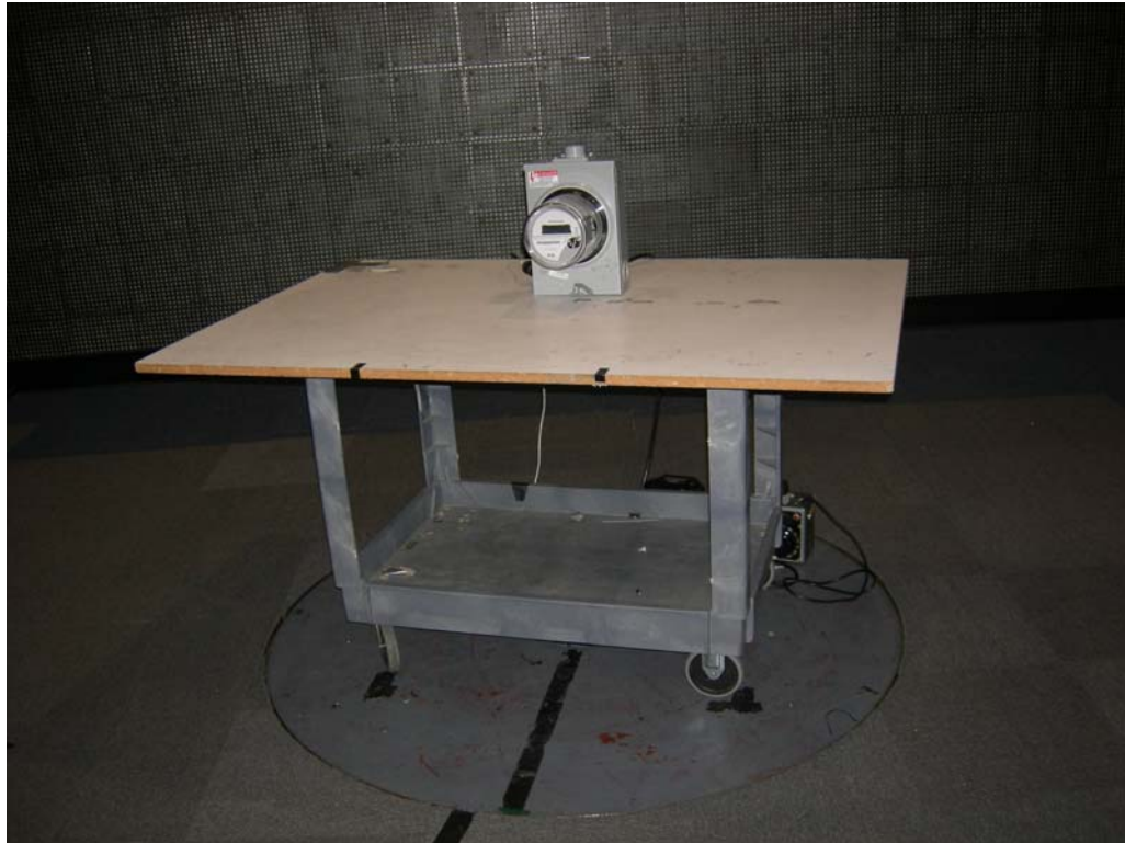
Figure 7: Test Setup – Radiated Emissions - Intentional
