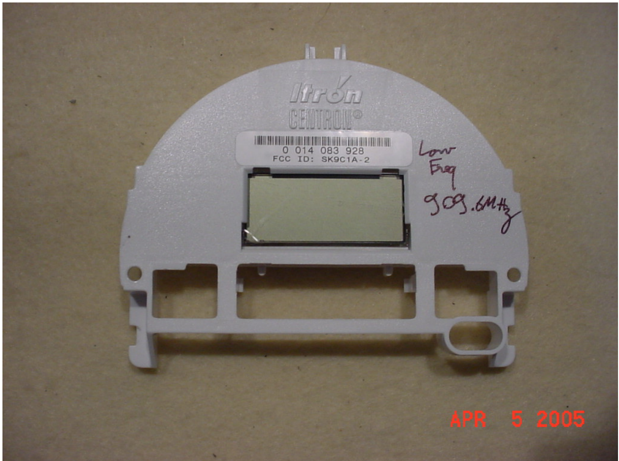
Figure 5: Meter Display Front View
