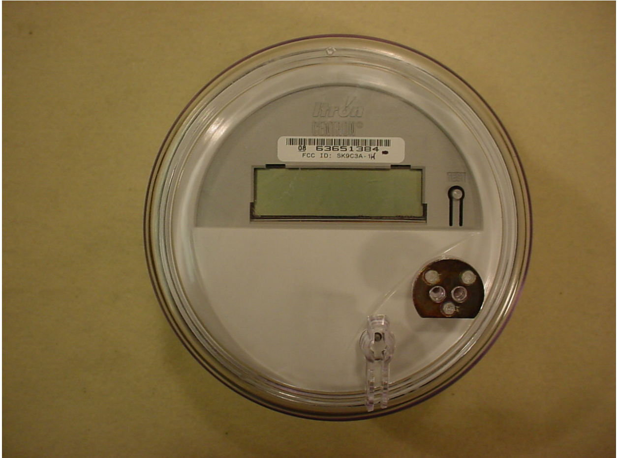
Figure 4: External – Front View - Polyphase Metrology Base
