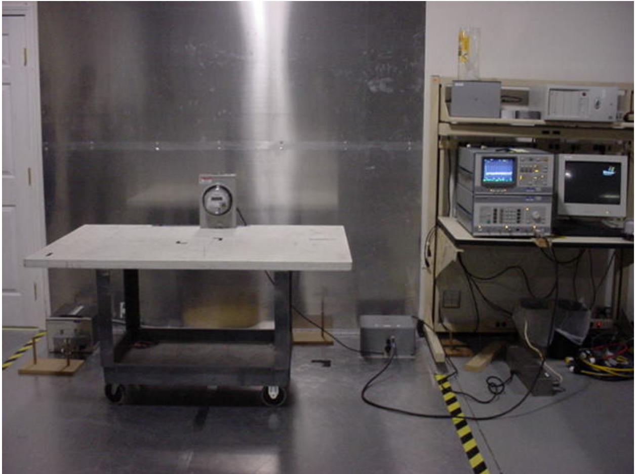
Figure 3: Test Setup – Conducted Emissions - Monophase
