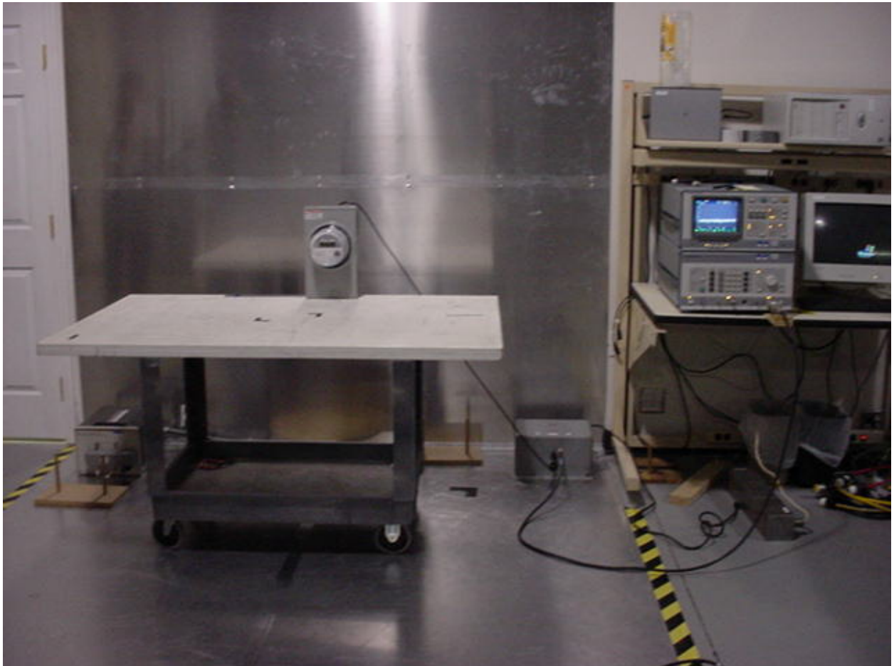
Figure 4: Test Setup – Conducted Emissions - Polyphase
