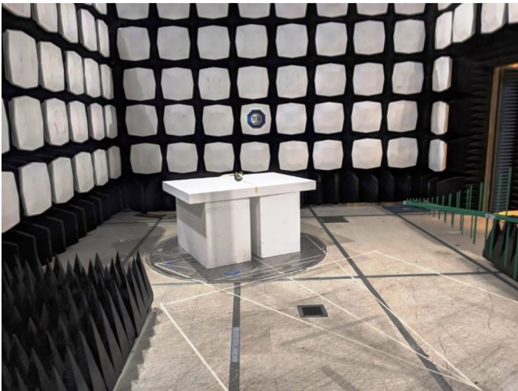
Figure 4: Equipment Under Test – Radiated Emissions <1GHz
