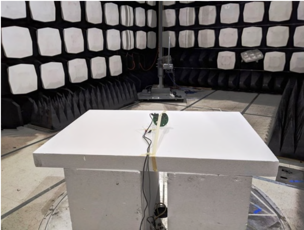
Figure 3: Equipment Under Test – Radiated Emissions <30MHz
