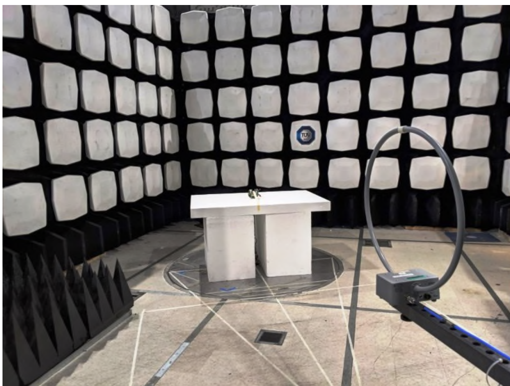
Figure 2: Equipment Under Test – Radiated Emissions <30MHz
