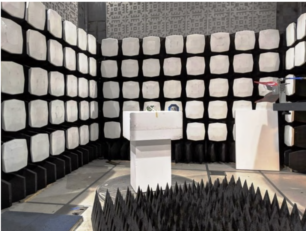
Figure 6: Equipment Under Test – Radiated Emissions >1GHz
