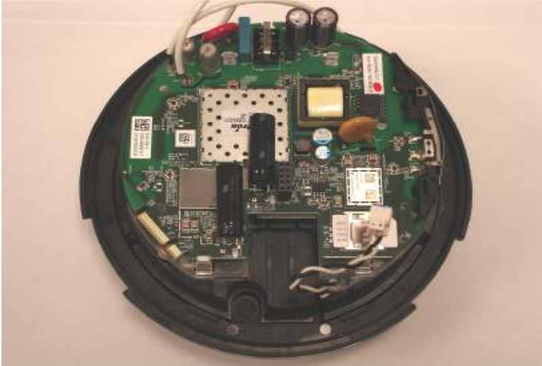
Meter Base with CAT1 and register boards installed
