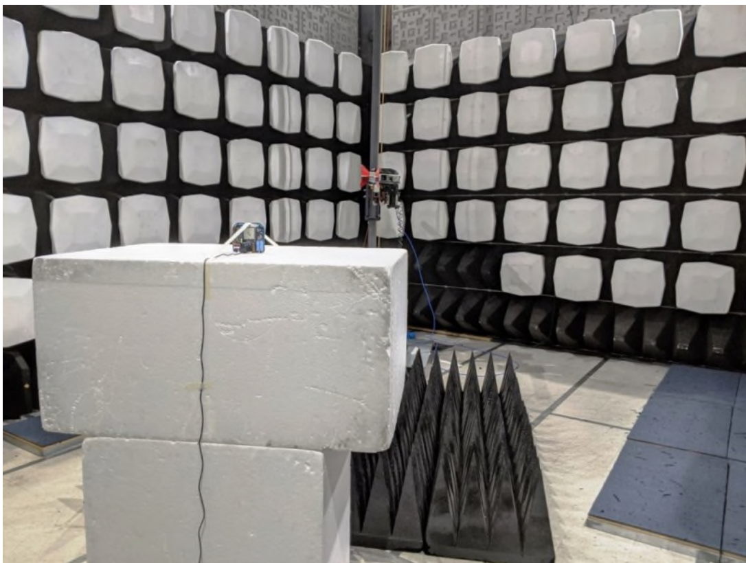
Figure 8: Test Setup – Radiated Emissions >1GHz
