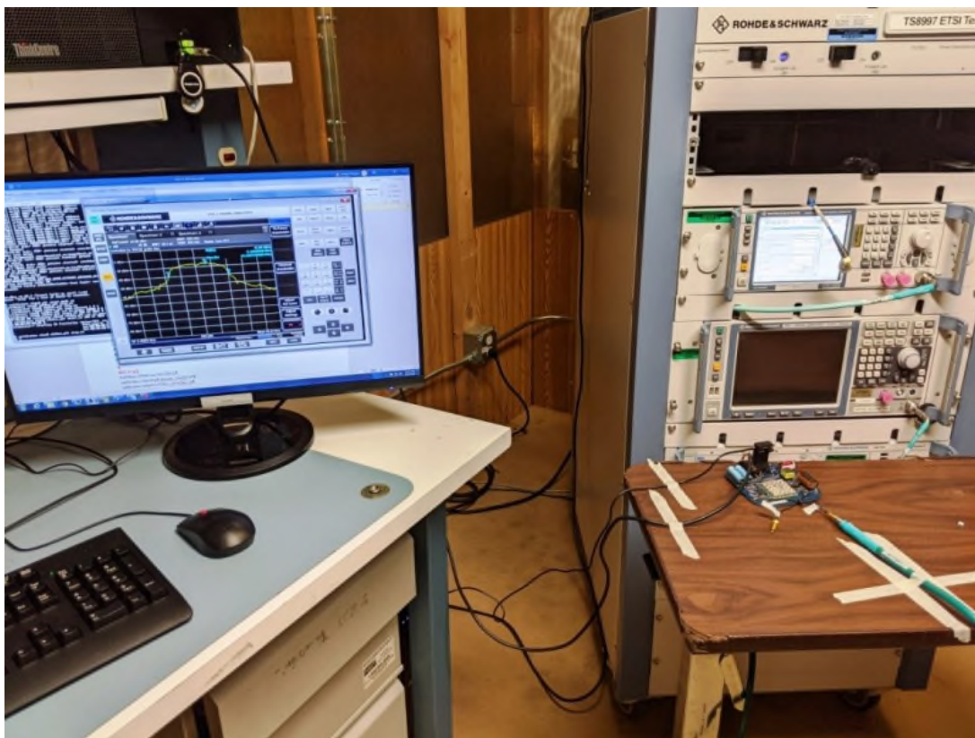
Figure 1: Test Setup –Antenna Port Conducted Measurements (WLAN)
