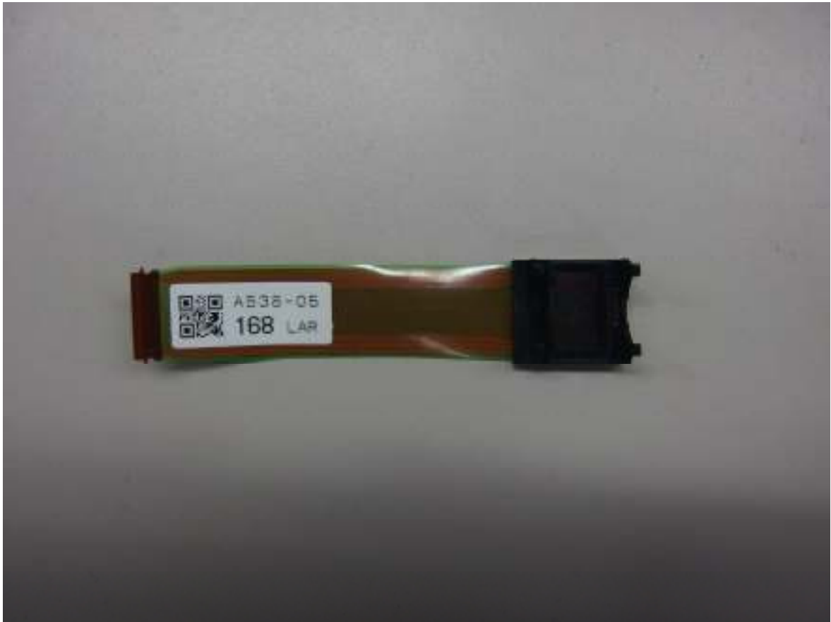
42. OLED Module L (surface)
