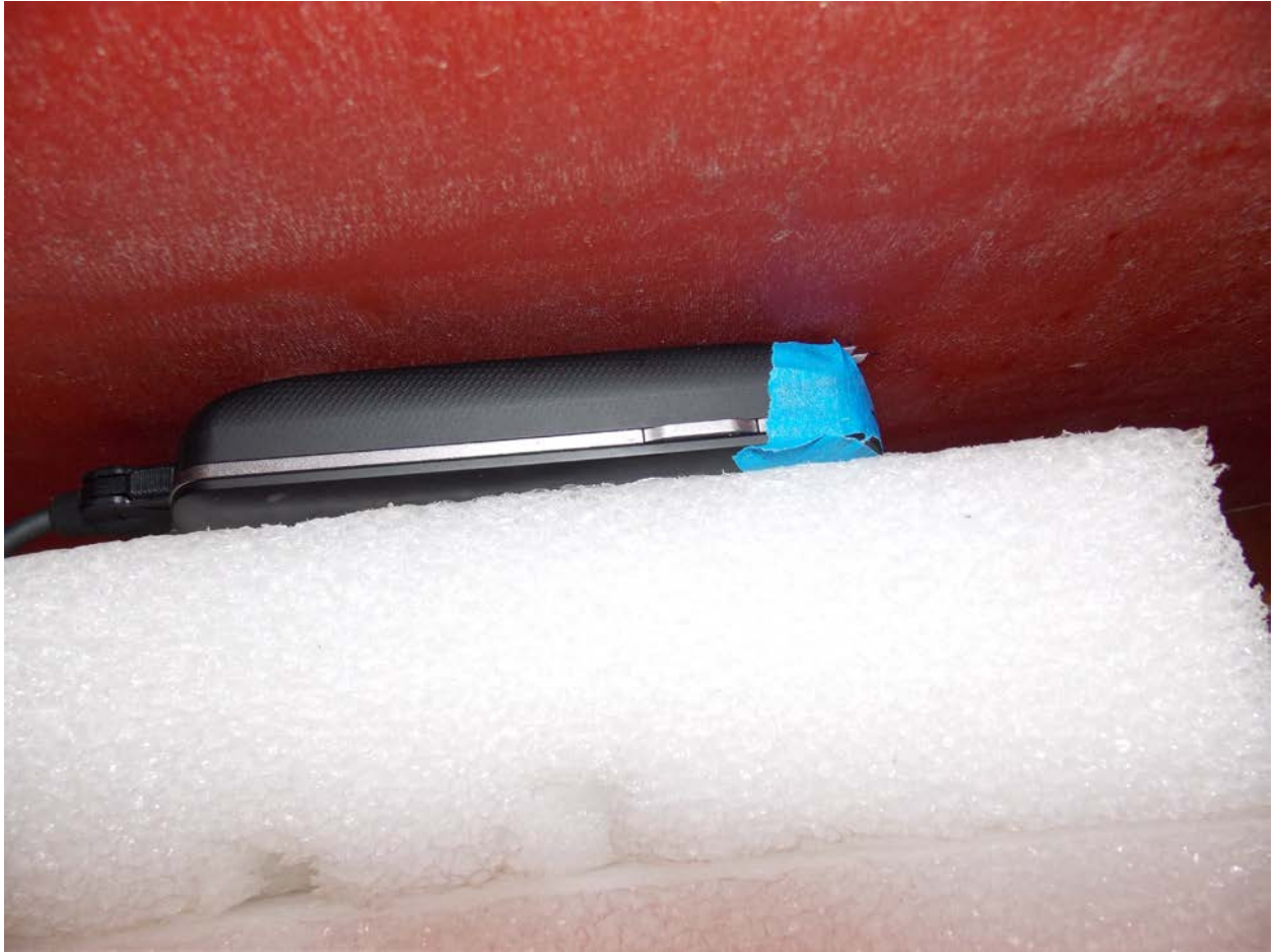
Test Position Back 0 mm Gap
