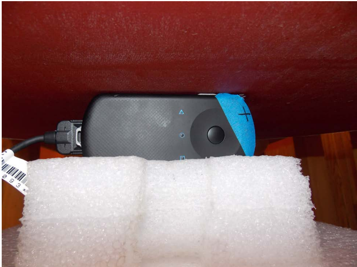
Test Position Left 0 mm Gap
