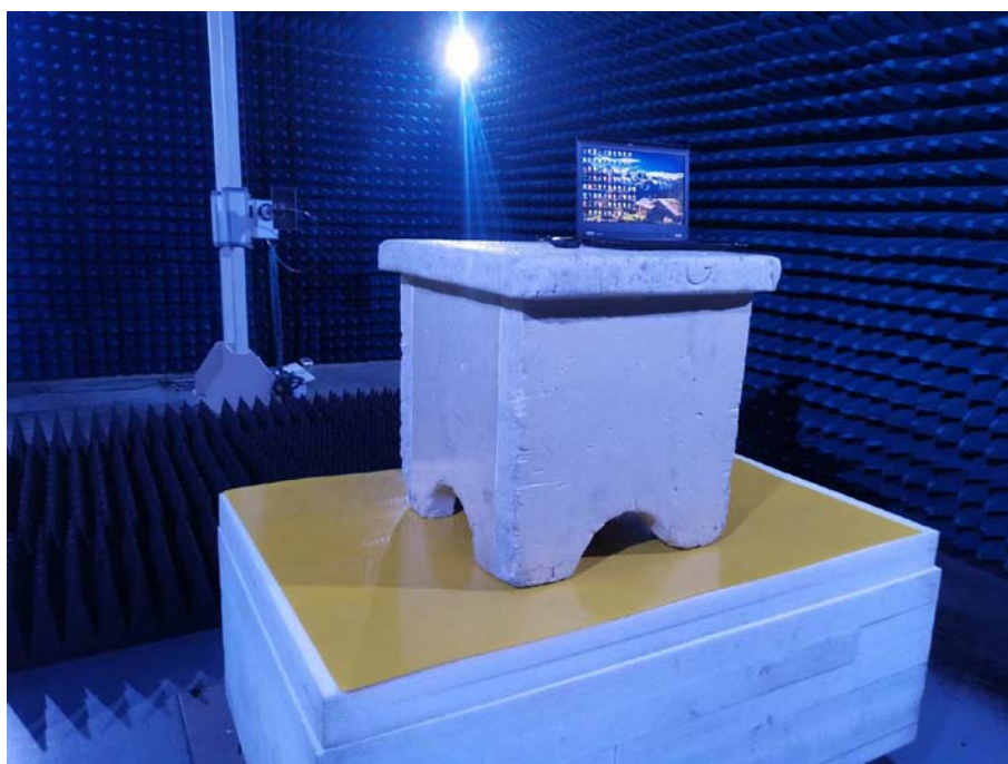
Photo of Radiated Emission Measurement Above 1GHz
