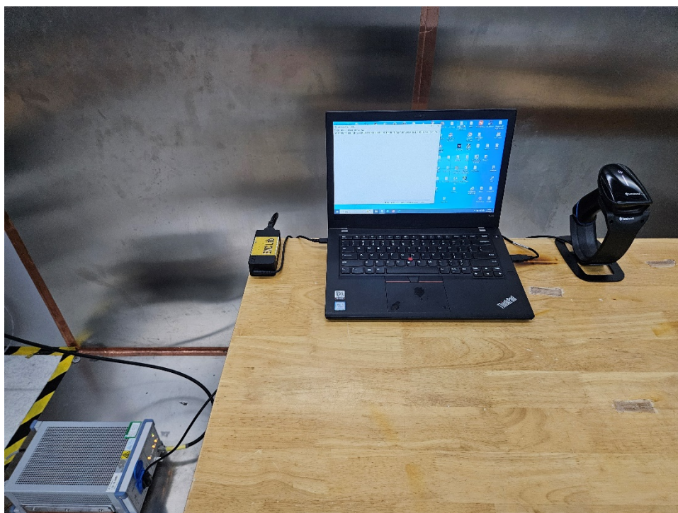
Photograph 3: Set-up for Conducted Emission on AC Mains
