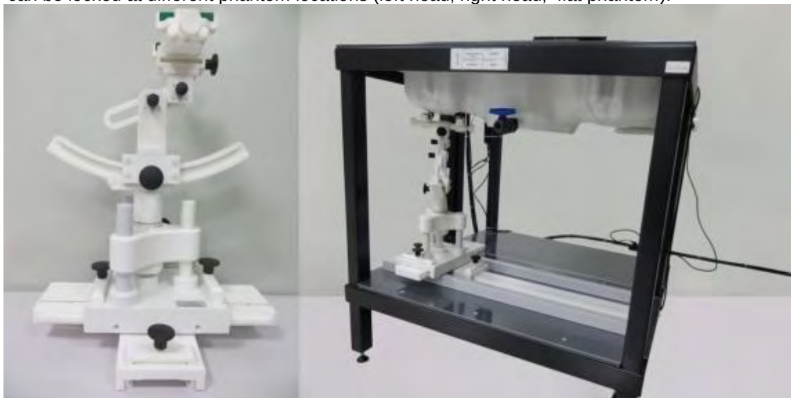
Device holder supplied by SATIMO
