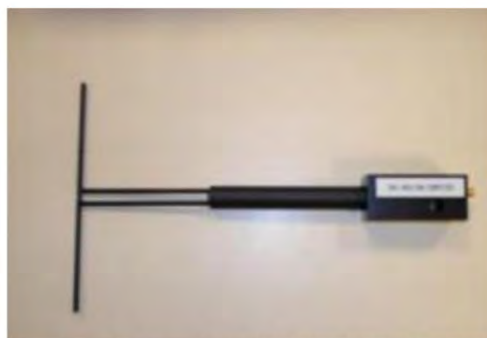
Figure 1 – Satimo COMOSAR Validation Dipole
