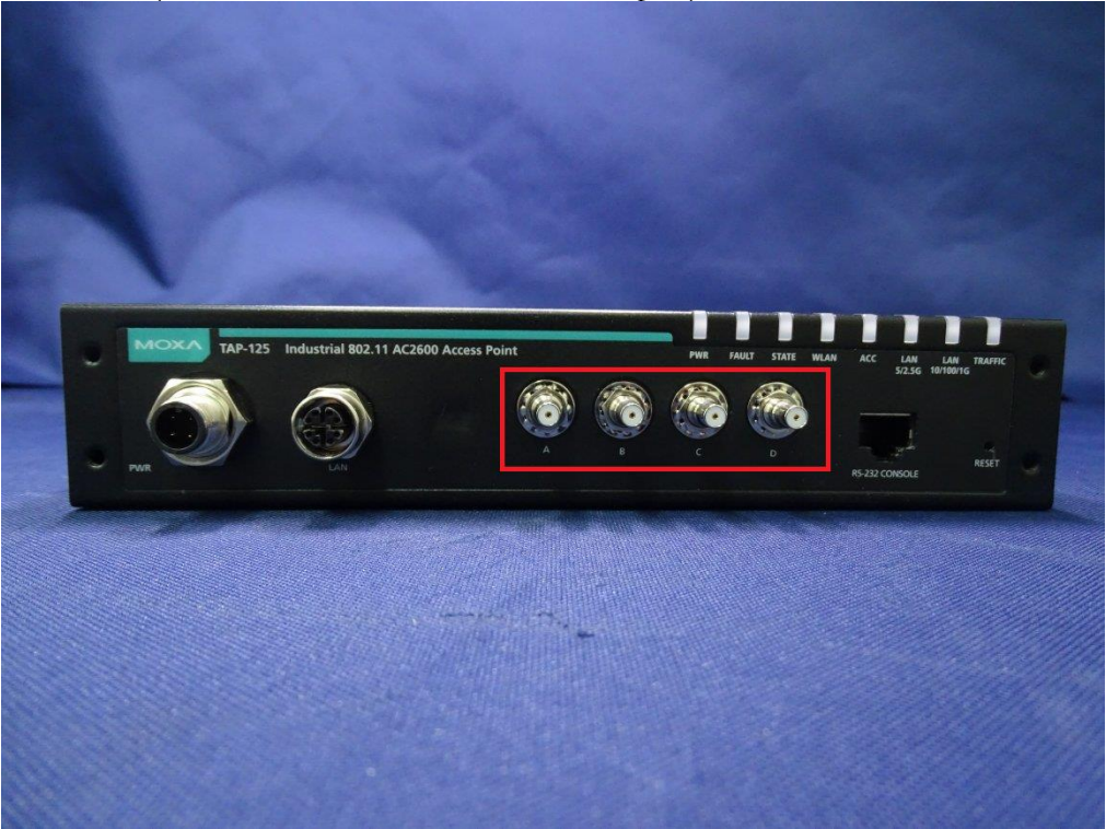
(3) EUT Photo (2.4GHz & 5GHz Antenna connector port)
