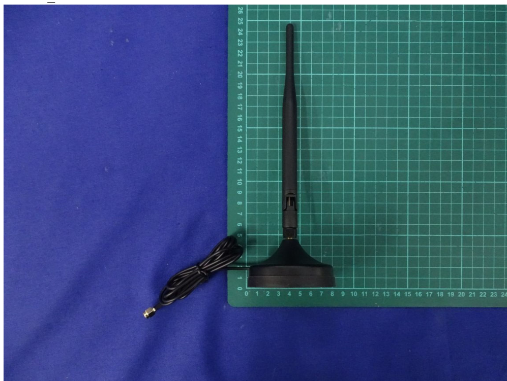
(29) EUT Photo_ Antenna: MOXA / ANT-WSB-AHRM-05-1.5m
