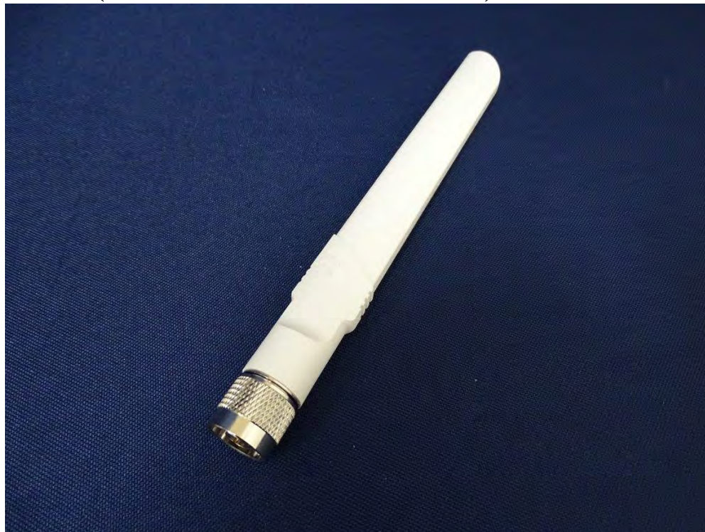
(7) EUT Photo (Antenna 1_ MOXA / ANT-WDB-ANM-0306)
