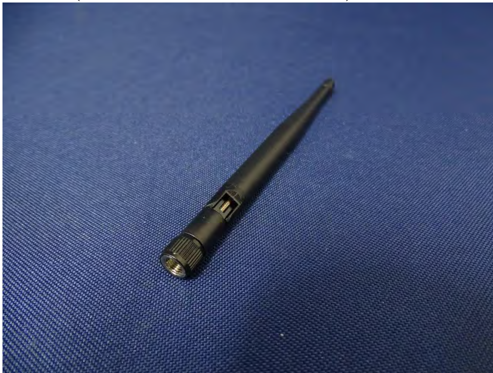
(15) EUT Photo (Antenna 4_ MOXA / ANT-WDB-ARM-0202)
