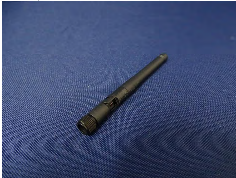
(23) EUT Photo (Antenna 6_ MOXA / ANT-WDB-ARM-02)
