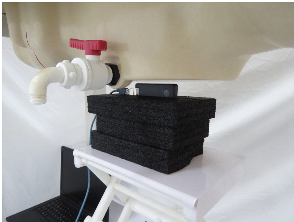
Picture 3: Left Edge, the distance from EUT to the bottom of the Phantom is 5mm
