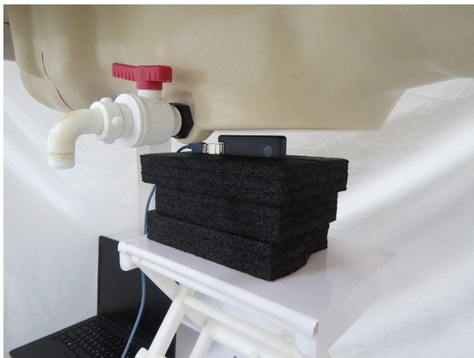
Picture 4: Right Edge, the distance from EUT to the bottom of the Phantom is 5mm
