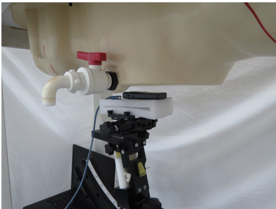
Picture 6: Back Side, the distance from EUT to the bottom of the Phantom is 16mm
