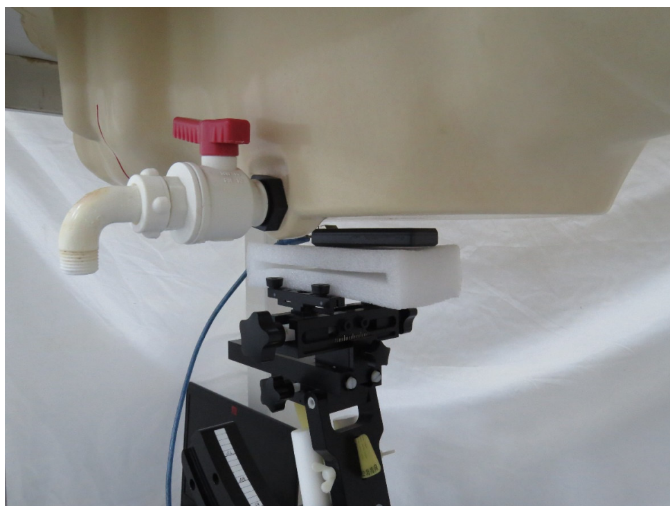
Picture 2: Front Side, the distance from EUT to the bottom of the Phantom is 5mm
