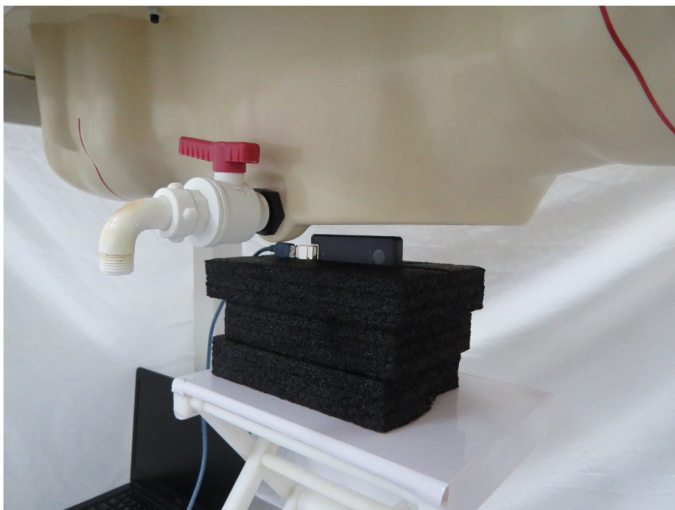
Picture 8: Left Edge, the distance from EUT to the bottom of the Phantom is 10mm
