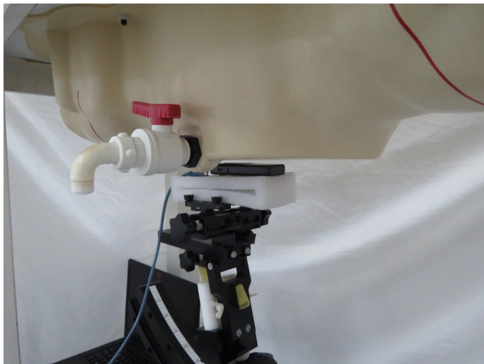
Picture 1: Back Side, the distance from EUT to the bottom of the Phantom is 5mm
