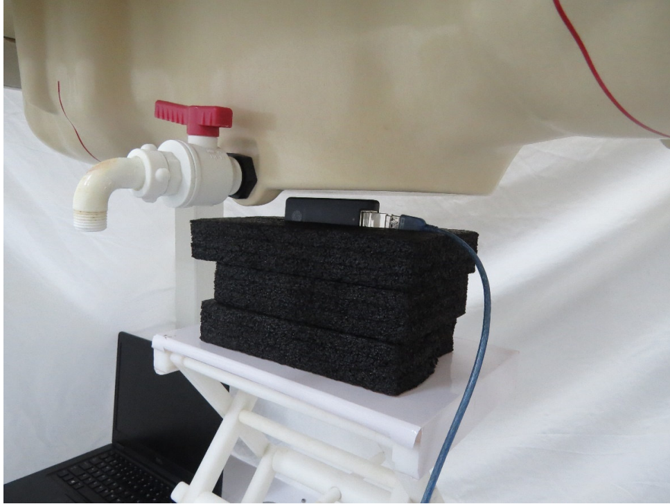
Picture 9: Right Edge, the distance from EUT to the bottom of the Phantom is 10mm
