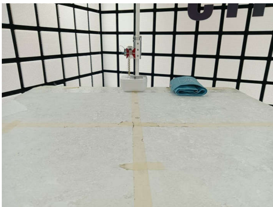
Radiated spurious emission Test Setup-2(Above 1GHz)
