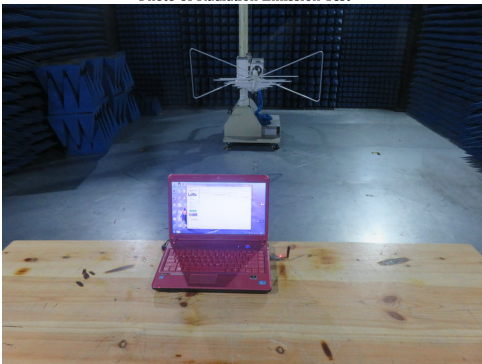
Photo of Radiation Emission Test
