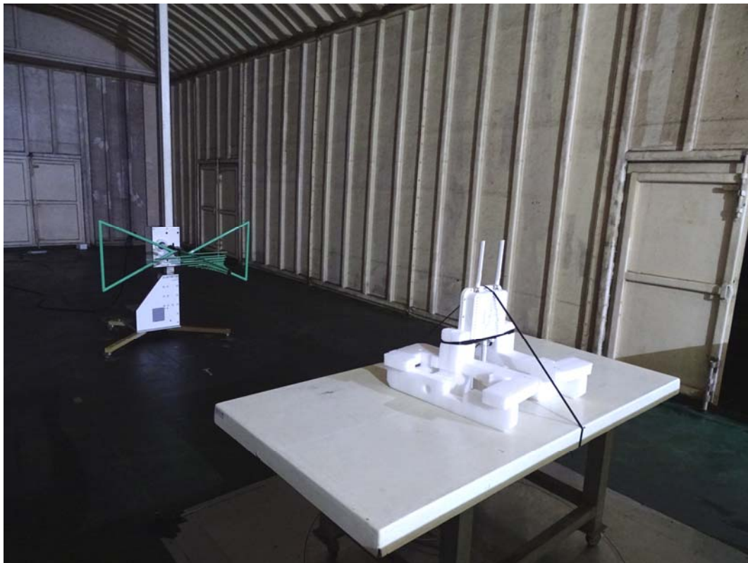
Back View of Radiated Test
