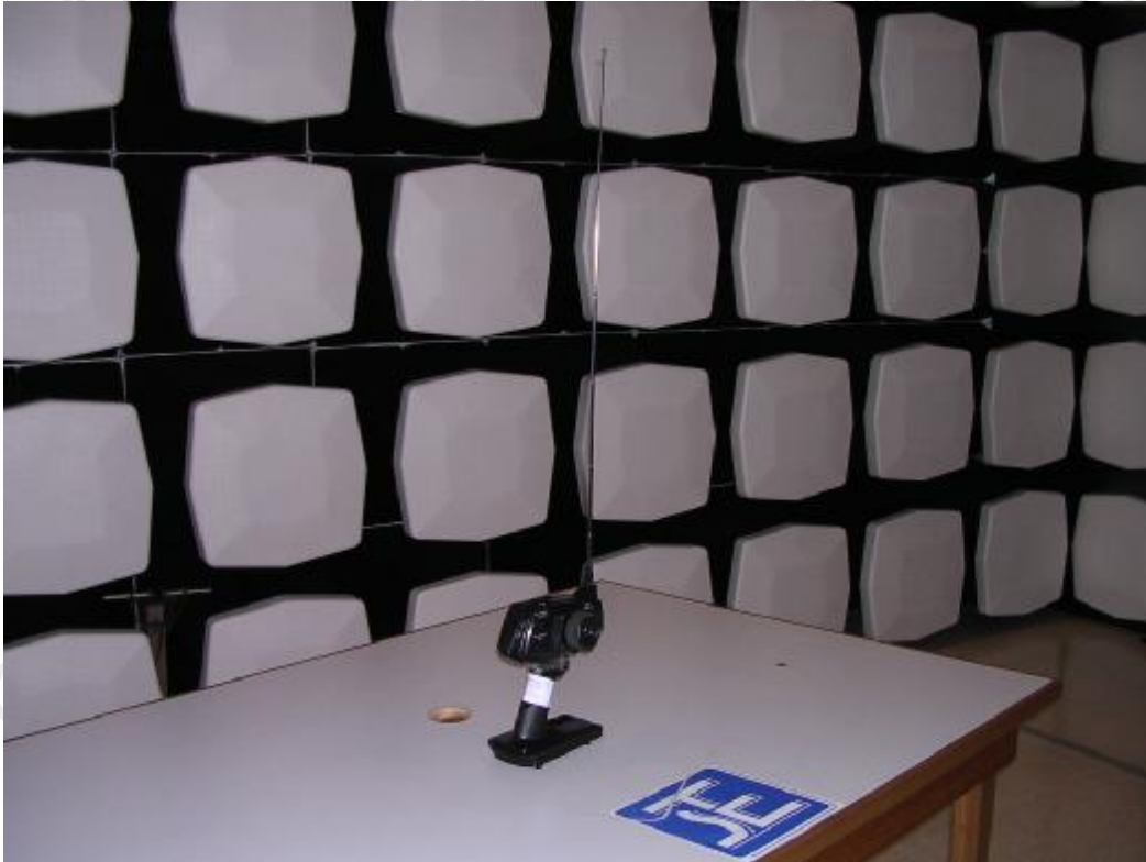
Measurement of Radiated Emission Test Set Up
