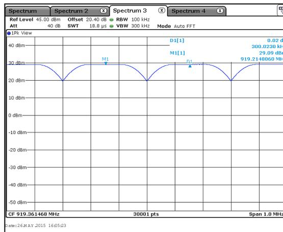
Figure 7.4.1.2-1: Carrier Frequency Separation 2604.2bps
