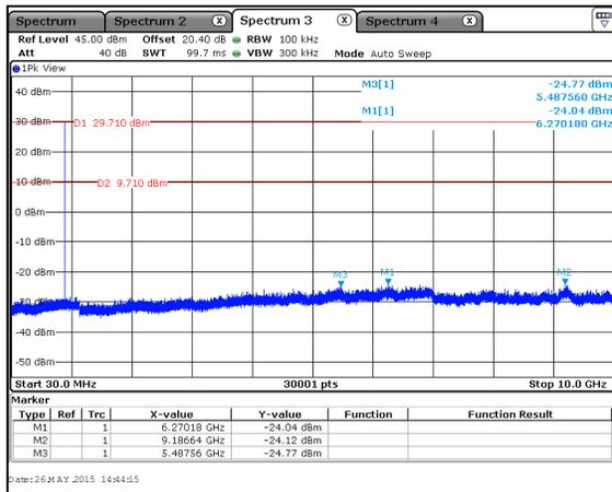
Figure 7.5.2.2-1: 30 MHz – 10 GHz – LCH 2604.2bps
