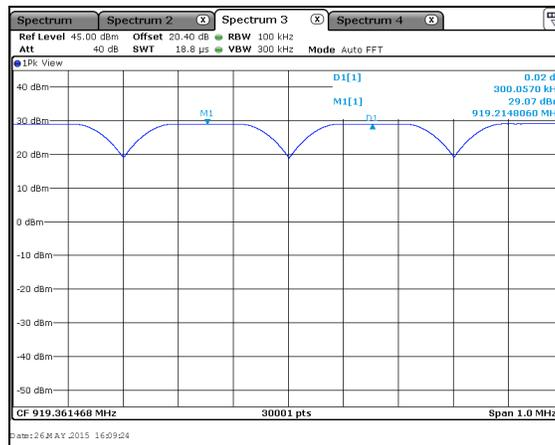
Figure 7.4.1.2-2: Carrier Frequency Separation 4557.3bps
