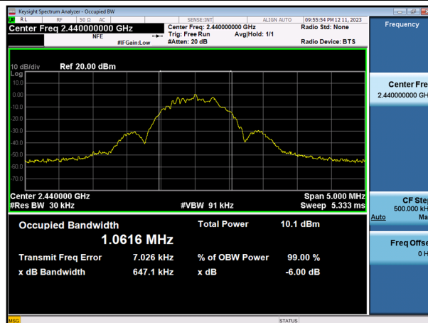
6 dB Bandwidth plot (High-CH 39)
