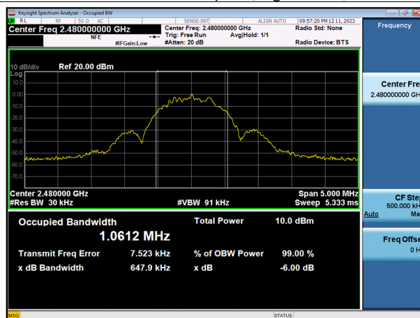
6 dB Bandwidth plot (High-CH 39)
