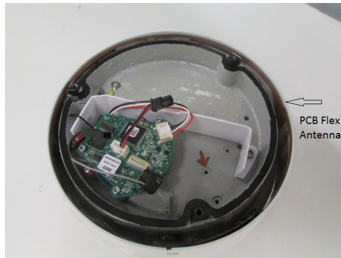
Figure 1: Module and Antenna installed in Host EchoShore - DX
