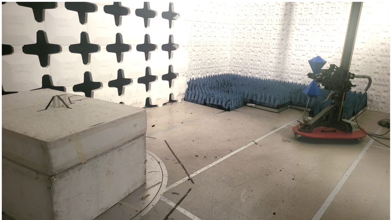
Figure 3. Radiated Emissions Test Setup (30 - 1000 MHz)
