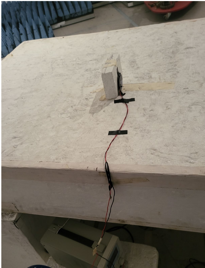
Figure 1. Radiated Emissions Test Setup
