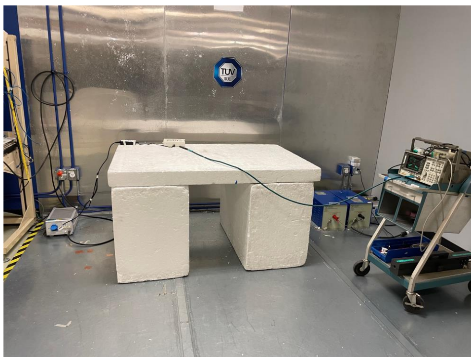
Figure 5: Test Setup – AC Power Line Conducted Emissions
