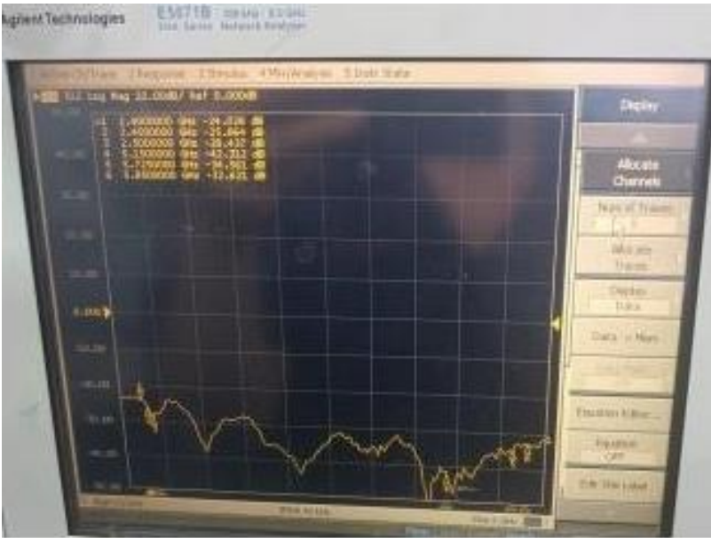
WIFI 1 and WIFI 2 isolation test diagram
