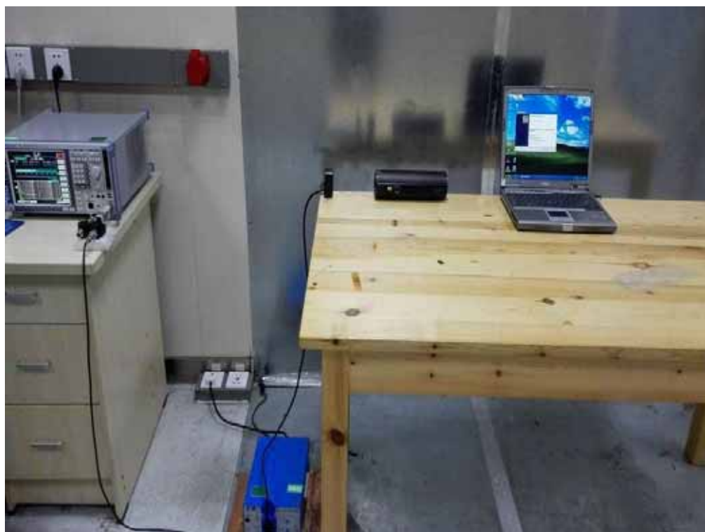
FCC RADIATED EMISSION TEST SETUP BELOW 1GHZ
