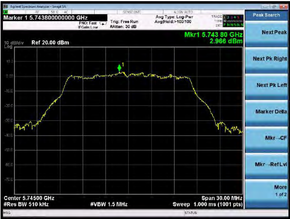
TEST PLOT OF SPECTRAL DENSITY FOR 5745MHz
