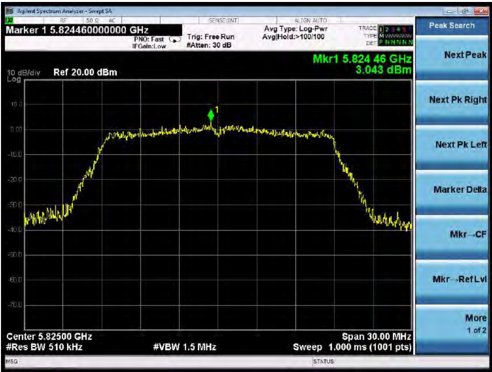
TEST PLOT OF SPECTRAL DENSITY FOR 5825MHz AT CHAIN 1
