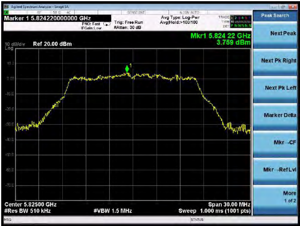
TEST PLOT OF SPECTRAL DENSITY FOR 5825MHz
