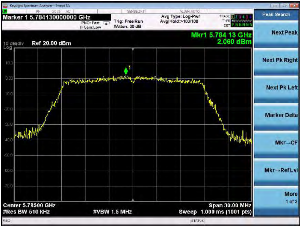
TEST PLOT OF SPECTRAL DENSITY FOR 5785MHz AT CHAIN 1
