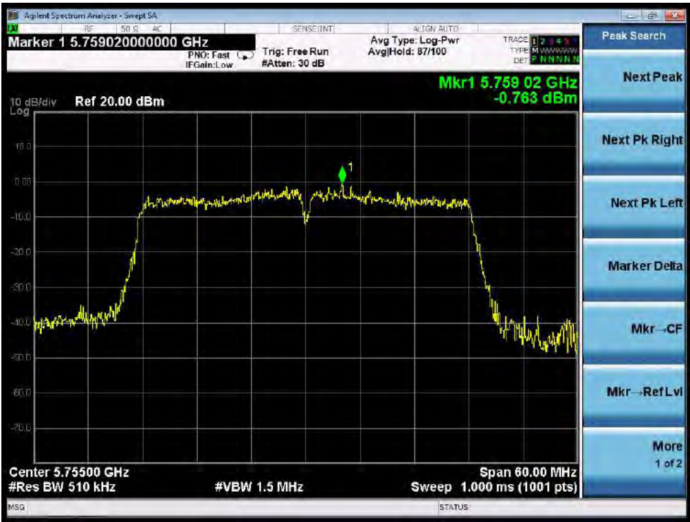
TEST PLOT OF SPECTRAL DENSITY FOR 5755MHz AT CHAIN 1
