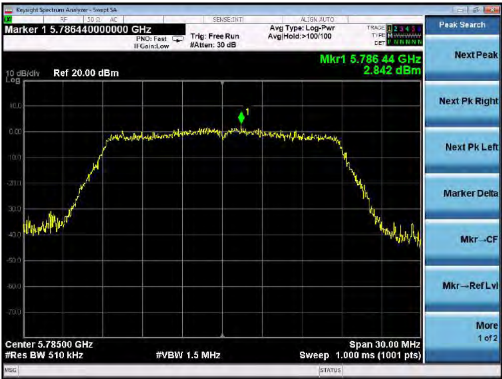
TEST PLOT OF SPECTRAL DENSITY FOR 5785MHz AT CHAIN 1
