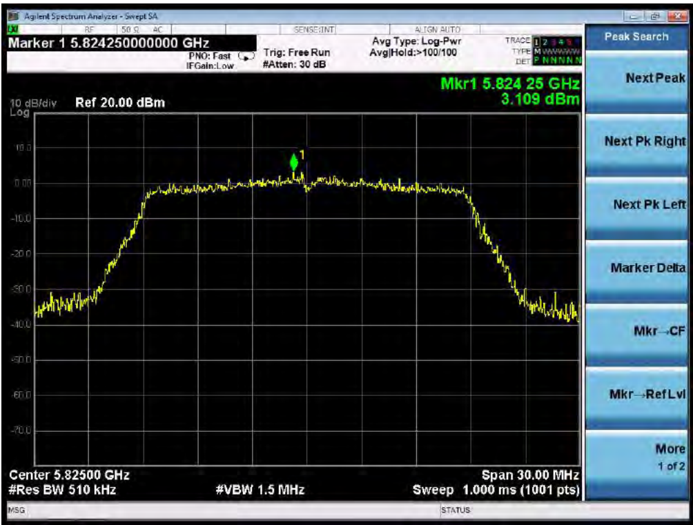
TEST PLOT OF SPECTRAL DENSITY FOR 5825MHz AT CHAIN 1
