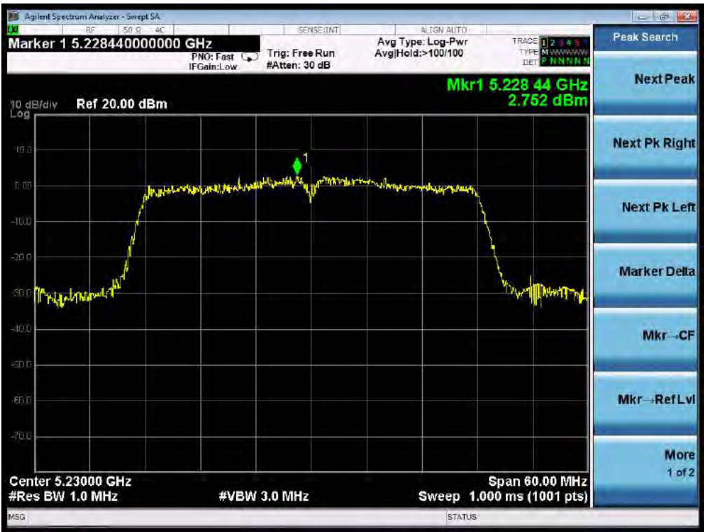
TEST PLOT OF SPECTRAL DENSITY FOR 5230MHz AT CHAIN 1
