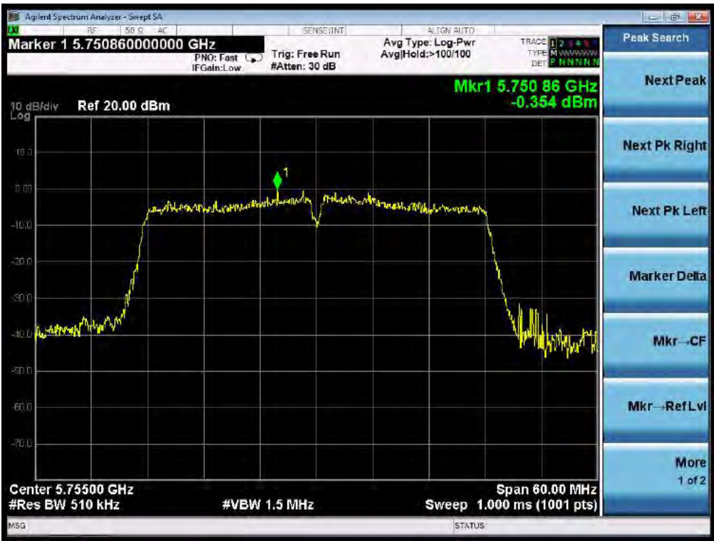
TEST PLOT OF SPECTRAL DENSITY FOR 5755MHz AT CHAIN 1
