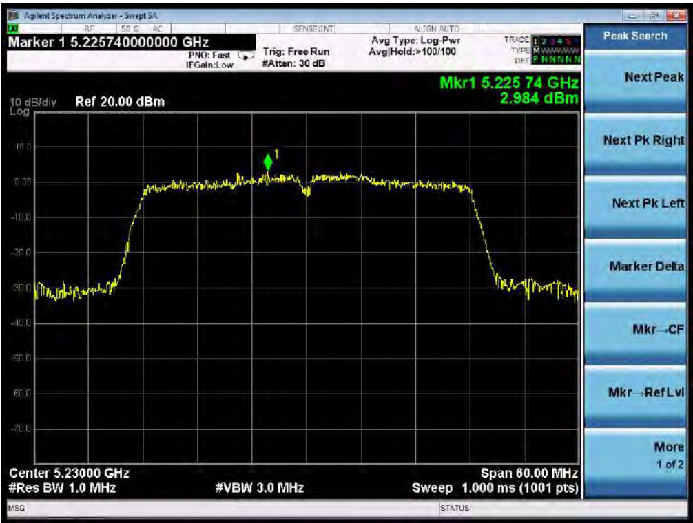
TEST PLOT OF SPECTRAL DENSITY FOR 5230MHz AT CHAIN 1
