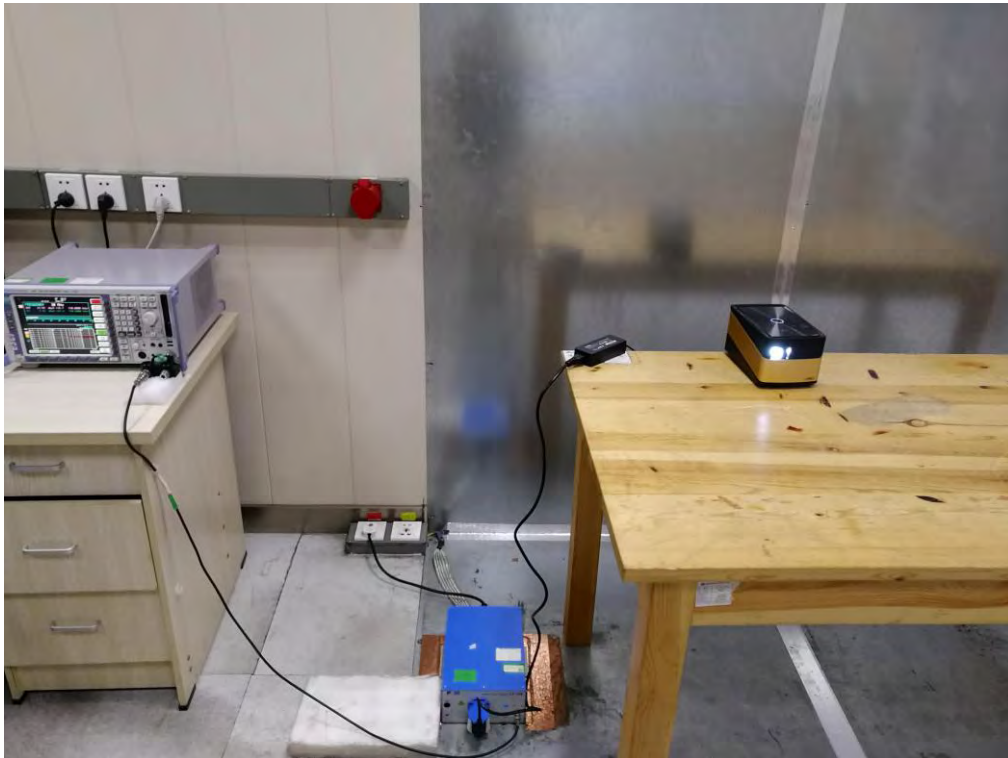
FCC RADIATED EMISSION TEST SETUP BELOW 1GHZ
