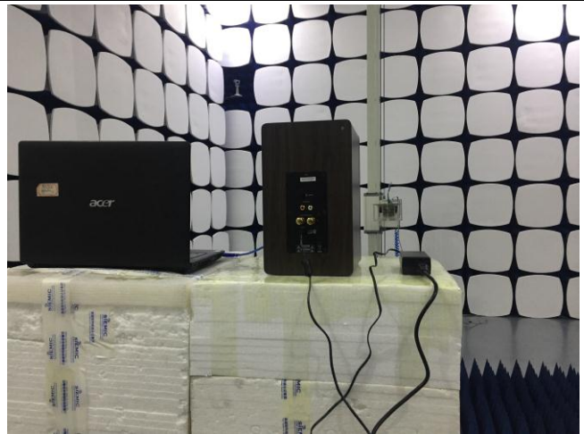
Radiated Spurious Emissions Test Setup Above 1GHz
