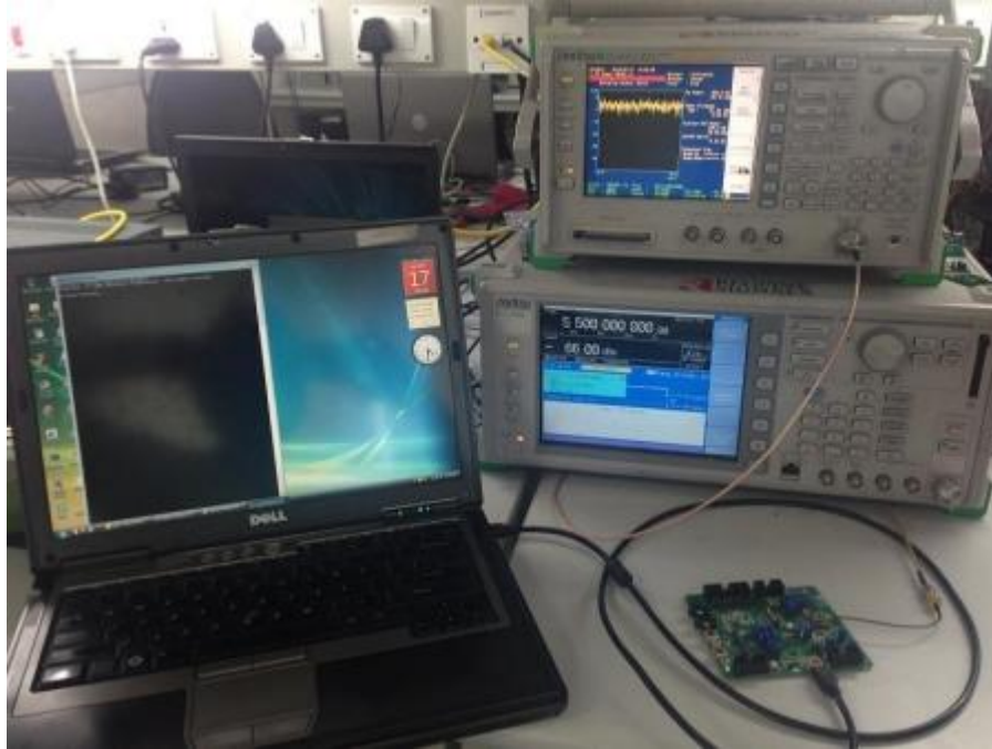
Figure 1: Linux Based RF Evaluation Setup With USB Interface
