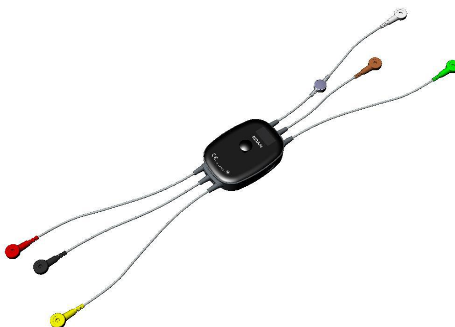
Figure 3-9 Wireless FECG Fetal&Maternal Module and ECG Leads
