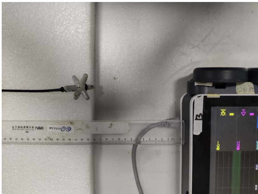
E-field Test Setup Photo of Position B(15cm)
