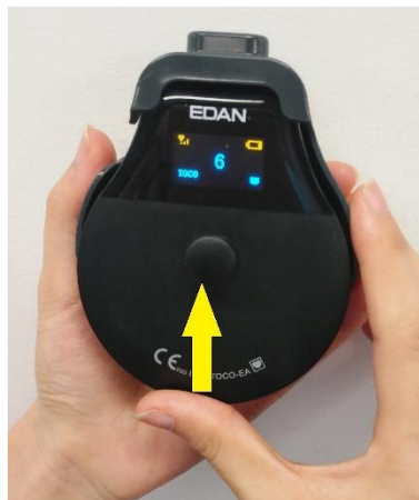
Figure 8-7 Install the Electrode Sleeve
