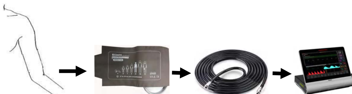
Figure 8-10 Connection for NIBP measurement
